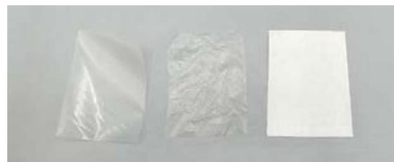
Sustratos probados, de izquierda a derecha: Aquatics Avalon 20 micron thick water soluble polyvinyl alcohol film, Aquatics Romeo 80 micron thick water soluble polyvinyl alcohol film, Sulky Paper Solvy water soluble paper 65% Cellulose and 35% Carboxymethyl cellulose.
